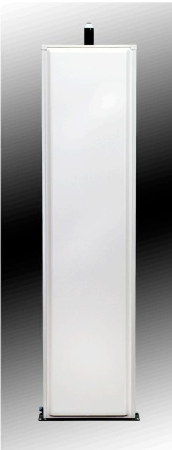
**THIN Portals™** come in two heights- 60" and 78", to cover a range of applications. The Reader Cabinets include two antenna brackets (but can fit up to 4 antennas), reader plate, white ABS cover, and reader power supply bracket. Unit comes with openings for 3/4" EMT conduit.
